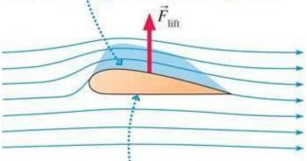
Because the pressure beneath the wing is higher than the pressure above, there's a net upward force on the wing. This is lift.
