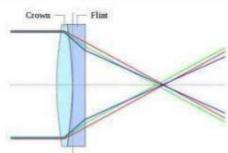
In a typical contact doublet the negative lens glass is about 1.5X to 2X more dispersive than the positive lens glass.
