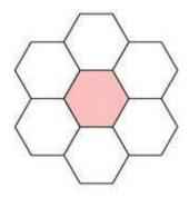
Here I will spread out as I/3 so when battery connected to adjacent nodes, the current in the resistance will be 2I/3 thus equivalent resistance will be 2R/3
