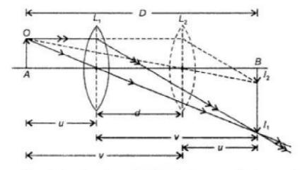
Let O be the size of object held perpendicular to the principal axis of the lens. A real, inverted and magnified image of size  $I_1$  is formed when the lens is at position  $L_1$ . When the lens is shifted to position  $L_2$  after moving to a distance  $d_1$  diminished image of size  $I_2$  is formed.
