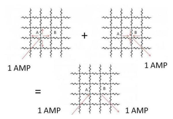
The principle of superposition says that if we add the two solutions we also get a solution. Adding the two configurations above means that the resistor joining A to B must be carrying 1/2 Amp (1/4 from the first solution and 1/4 from the second, both in the same direction). But this is a  $1\Omega$  resistor so the Voltage across AB must be 1/2 V.
