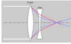
The color of a positive lens can be cancelled by an equal power negative lens of the same glass, but then the focal length of the lens pair would be zero, if they were in contact. Instead we want the negative lens to be a more dispersive glass than the positive lens, so that a weaker power negative lens can still cancel out the color and give a total power of the lens pair that is not zero. When the red and blue light rays come to the same focus primary color has been corrected.
