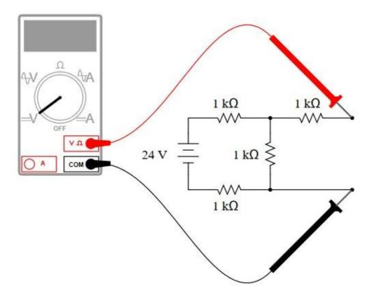
Next, calculate the current seen at the load terminals with an ammeter directly connected across them (a short-circuit condition)
