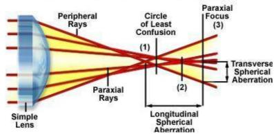
Optics - 8 ) Aspherical lenses can be used to reduce axial spread (of paraxial rays), apart from stoppers or rather with combinations of stoppers.
