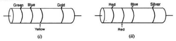
Solution. The first colour represents the digit 5. The second colour represents the digit 6. The third colour represents the digit 4, *i.e.*, four zeros. Therefore, the value of the resistance is  $56,0000 \Omega$ . The fourth gold strip indicates  $\pm 5\%$  tolerance. Hence, resistance specification of the resistor is
