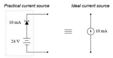
The current-limiting diode acts as a variable resistance, to regulate current through it at a constant value: if current increases, its resistance increases to reduce the current back to where it should be; if current decreases, its resistance decreases to increase current up to where it should be.
