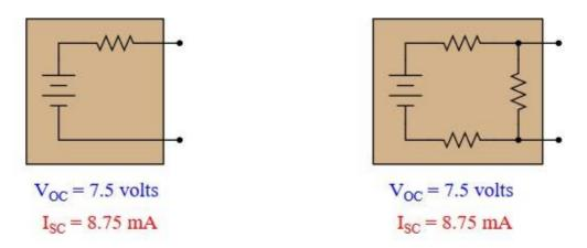
With equal  $V_{OC}$  and  $I_{SC}$  figures and with linear componentry, the load lines must be identical. This means that any load resistance, when connected to each of the power sources, will experience the exact same voltage and current.
