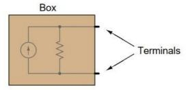
How would you experimentally determine the current of the ideal current source inside this box, and how would you experimentally determine the resistance of the parallel resistor? By "experimentally," I mean determine current and resistance using actual test equipment rather than assuming certain component values (remember, this "black box" is sealed, so you cannot look inside!).
