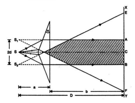
In a biprism experiment, the eye-piece was placed at a distance of 120 cm from the source. The distance between two virtual images was found equal to 0.075 cm. Find the wavelength of light of source if eye-piece is moved through a distance of 1.888 cm for 20 fringes to cross the field of view.
