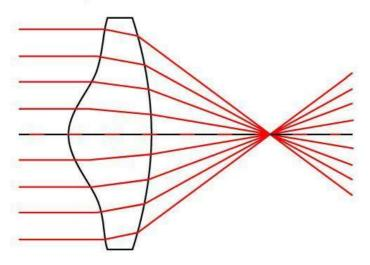
Remember more curved surface should face the light first. In plano-convex lens the convex part should face the light for better utilization of refraction properties. Also this minimizes the errors.
