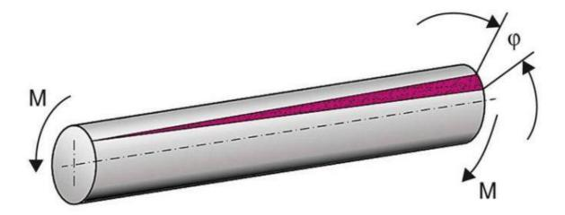
The torque T can be equated to the sum of the moments of the tangential stresses on the element  $2\,\pi\,r\,\delta r$
