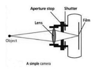
If  $n_1$  and  $n_2$  are f-numbers of two cameras and  $t_1$  and  $t_2$  are the exposure times then (  $t_1 / t_2$  ) = (  $n_1 / n_2$  )<sup>2</sup>
