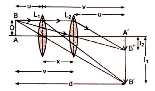
(ii) Here,  $I_1$  and  $I_2$  are the lengths of images in first and second position of lens L. O is the length of the object. In first position of lens,
