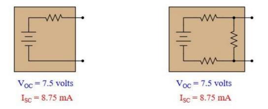
With equal  $V_{OC}$  and  $I_{SC}$  figures and with linear componentry, the load lines must be identical. This means that *any* load resistance, when connected to each of the power sources, will experience the exact same voltage and current.
