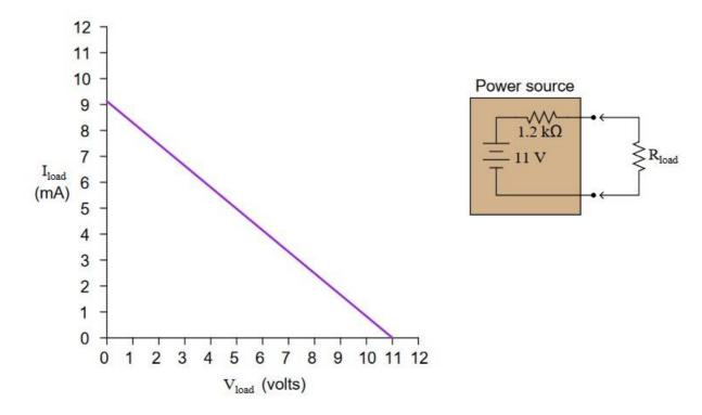
Hint: the easiest points on find on this load line are the points representing open-circuit and short-circuit conditions (i.e.  $R_{load} = \infty \Omega$  and  $R_{load} = 0 \Omega$ , respectively).
