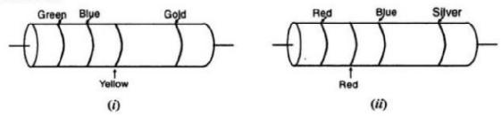
Solution. The first colour represents the digit 5. The second colour represents the digit 6. The third colour represents the digit 4, *i.e.*, four zeros. Therefore, the value of the resistance is 56,0000  $\Omega$ . The fourth gold strip indicates ± 5% tolerance. Hence, resistance specification of the resistor is
