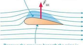
Because the pressure beneath the wing is higher than the pressure above, there's a net upward force on the wing. This is lift.
