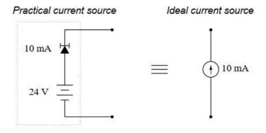
The current-limiting diode acts as a variable resistance, to regulate current through it at a constant value: if current increases, its resistance increases to reduce the current back to where it should be; if current decreases, its resistance decreases to increase current up to where it should be.
