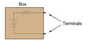
How would you experimentally determine the voltage of the ideal voltage source inside this box, and how would you experimentally determine the resistance of the series resistor? By "experimentally," I mean determine voltage and resistance using actual test equipment rather than assuming certain component values (remember, this "black box" is sealed, so you cannot look inside!).
