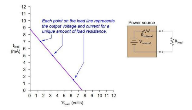
Note how the load line shows the voltage "sag" of the power source in relation to the amount of current drawn by the load. At high currents, the output voltage will be very low (upper-left end of load line). At low currents, the output voltage will be near its maximum (lower-right end of load line). If all internal components of the power source are *linear* in nature, the load line will always be perfectly straight.
