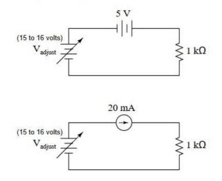
A practical *current source* may be built using a battery and a special semiconductor component known as a *current-limiting diode*:
