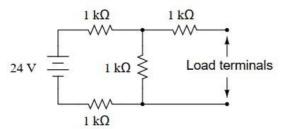
First, calculate the voltage seen at the load terminals with a voltmeter directly connected across them (an open-circuit condition)
