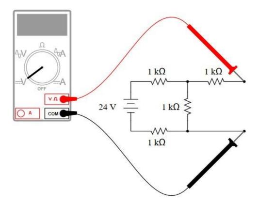
Next, calculate the current seen at the load terminals with an ammeter directly connected across them (a short-circuit condition)
