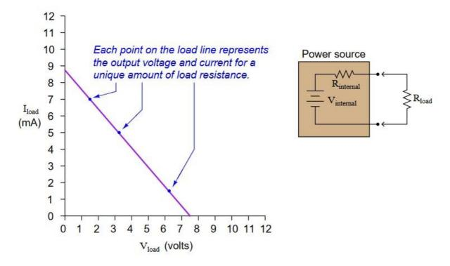
If we know that all the internal components of a power source are inherently *linear*, we know that the load line plot will indeed by a straight line. And, if we know the plot will be a straight line, all we need in order to plot a complete load line are *two* data points.
