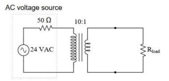
Equivalent source voltage = 2.4 VAC; equivalent source resistance =  $0.5 \Omega$ .
